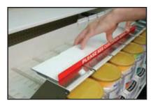
Remove the night lockout bars (if applicable), from the front of the shelf and place them on the plastic extrusion in the rear of the drawer.
